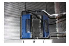
Place the machine on the first step and start the machine by lowering the handle. Start the escalator or motorized walkway. Preferably so that it is moving towards the operator. It is important for all three stabilizing guiding wheels to be inserted into the same channel or track, otherwise the machine could move sideways and work in an irregular manner.
